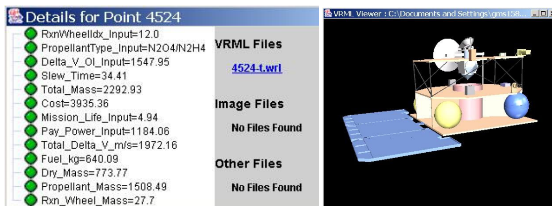
Figure 4-6: Quantitative Information and 3D Geometry of a Selected Point Design
