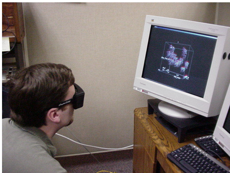
Figure 2-11: Active Stereoscopic Visualization Using LCD Shutter Glasses
