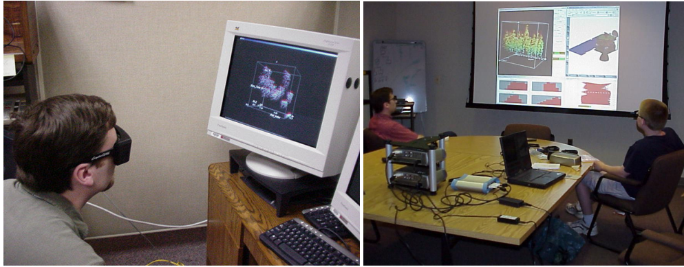
Figure 4. Active and Passive Stereoscopic Display. 1,2
